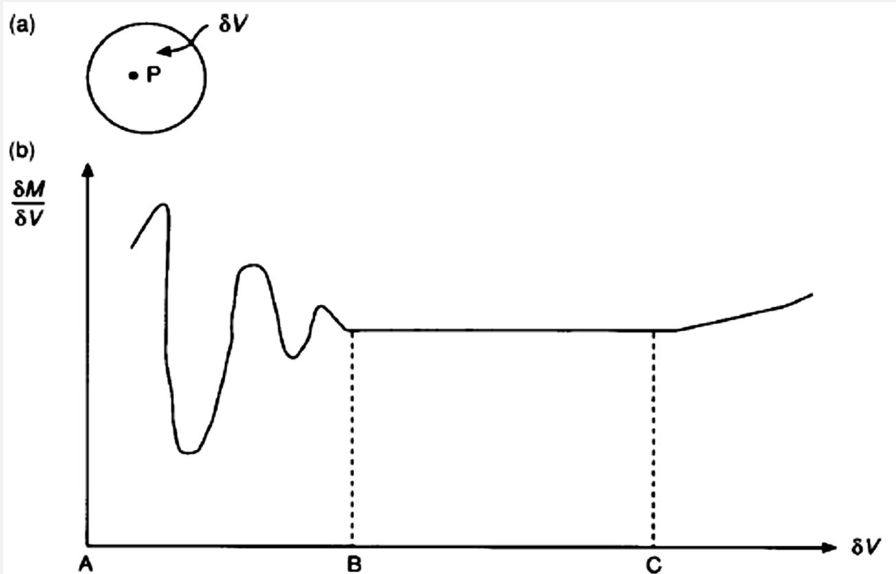
*Figure 5.3* Definition of the density  $\rho$  at a point  $P$  in a fluid
